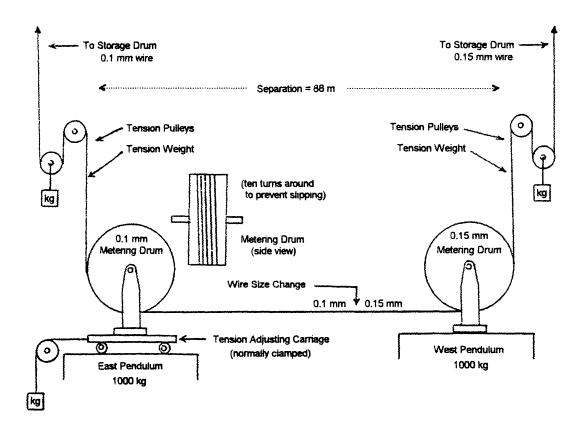
Figure 1. Schematic of a very low frequency (VLF) gravity wave antenna.
