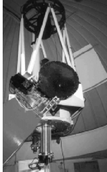
Figure 1. The MJUO Optical Craftsman 0.6m telescope. The long cylinder at the back end of the telescope is the focal reducer, with the SBIG ST-9e camera below it.
