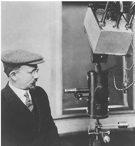
Figure 6. Dr. Joel Stebbins at Washburn Observatory, University of Wisconsin, about 1924. The telescope is a 15.3-inch Clark refractor. The photometer is possibly an early gimbal-mounted string electrometer.
