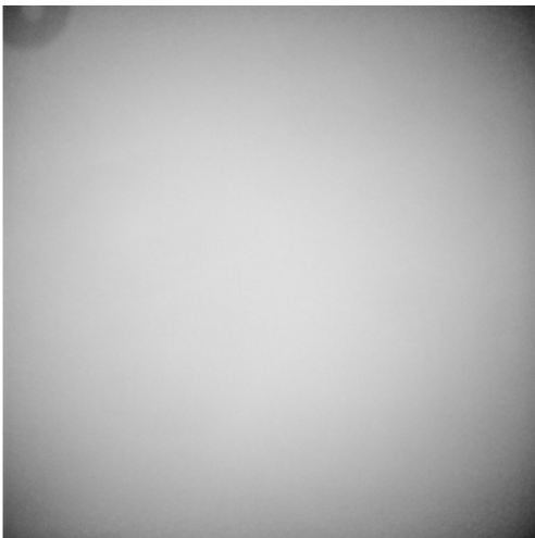
Figure 9. A master flat field obtained in the V filter, created from the median combination of multiple twilight flats.
