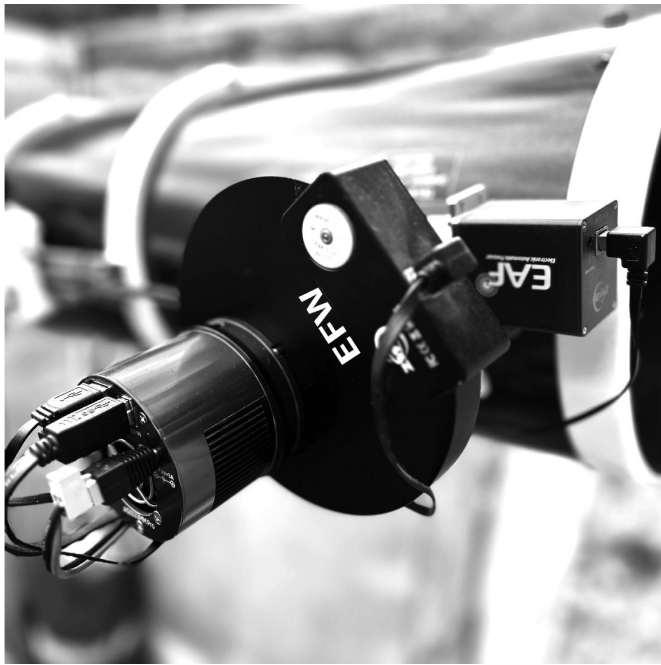
Figure 3. Camera ASI533 MM Pro CMOS, filter wheel, and automatic focuser mounted on the 0.25-m telescope.
