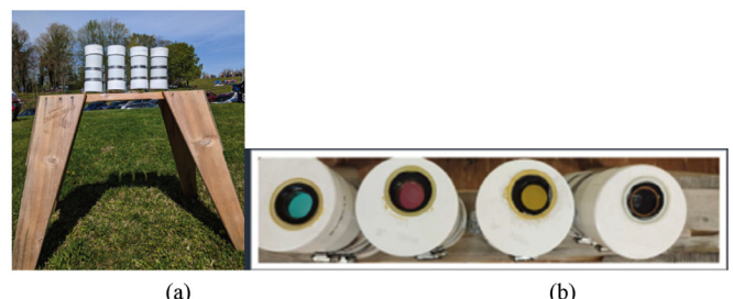
Figure 1. (a) Bank of SQM-L-DL devices in weatherproof housing and mounted on a sawhorse viewed from the side. (b) A view from the top with filters visible, from left to right: Red (R), Green (G), Blue (B), and clear or luminous (L).
