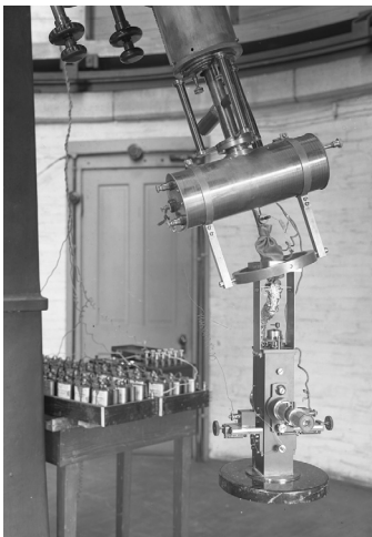
Figure 5. The photometer Stebbins used from about 1915 at the UI Observatory. The photometer contains a Kunz rubidium cell with a direct connection to a string electrometer specifically built for Stebbins by William Gaertner and Company of Chicago. The other parts were constructed by Mr. J. B. Hayes, mechanic of the Illinois physics department. The telescope is the UI 12-inch Brashear refractor. Provided by M. Svec, courtesy of University of Illinois Archives.
