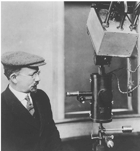
Figure 6. Dr. Joel Stebbins at Washburn Observatory, University of Wisconsin, about 1924. The telescope is a 15.3-inch Clark refractor. The photometer is possibly an early gimbal-mounted string electrometer.
