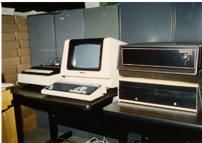
Figure 3. The Ithaca-Intersystems computer at AAVSO's Concord Street Headquarters, early 1980s. The system brought AAVSO's data processing operations in-house. Some of the hundreds of boxes of punch cards can be seen on the left, forming a work-area partition.
