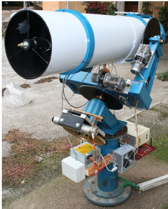
Figure 1. Observations were obtained using this homemade 255-mm F/4.7 Newton telescope, equipped with Starlight Xpress Trius-SX9 CCD camera, with a sensor area of 1392 × 1040 pixels (Pixel size: 6.45 × 6.45 μM).
