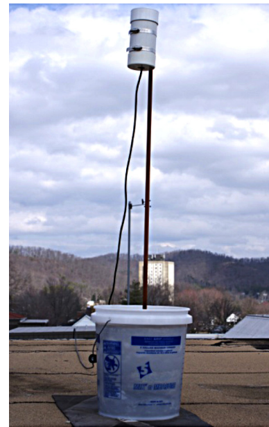
Figure 4. An example SQM-LE installation; this is the Morehead, Kentucky site. It is located on the roof of a four-story building located away from light sources and shadowing from trees or buildings. The device is pointed at zenith.
