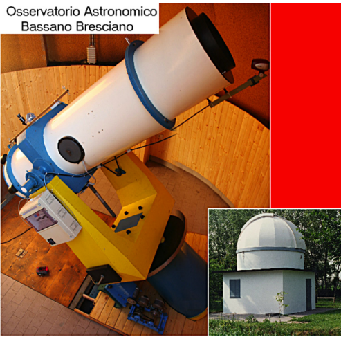
Figure 1. Observations were obtained using home-made 0.4-m Schmidt telescope operating at an effective focal ratio of f/10 , equipped with Starlight Xpress Trius-SX9 CCD.
